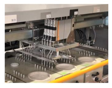
from black to white color. The system demonstrates a high level of automation and a coating efficiency of 95% or more.
