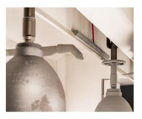
requirement for fully uniform layer thickness distribution. Accurate distribution is a must to ensure that the markings and characters on each type of gas cylinder remain perfectly legible after the burning-in process.
