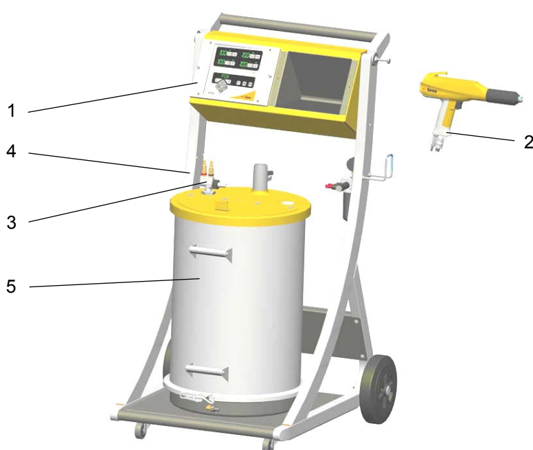
OptiFlex F manual coating equipment - structure
